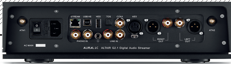
ABOVE: Wired/wireless network control/streaming supplements access to more music via internal and external (HDD) USB-A drives. A USB-B (DSD512/DXD) input is joined by Toslink, coax and AES (DSD64/192kHz) alongside analogue line and phono inputs. Variable analogue output is on RCAs and balanced XLRs
