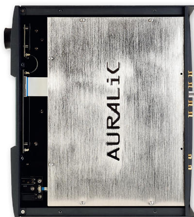
ABOVE: Hidden under the top-plate and screening the digital electronics within is a branded, silver-coloured enclosure
