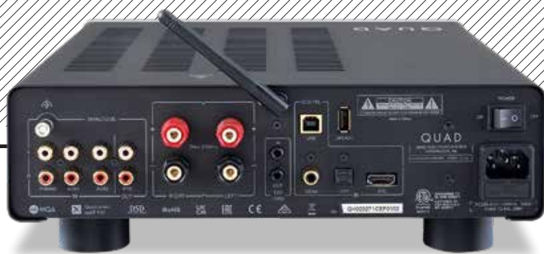
ABOVE: One MM phono and two line inputs are joined by a preamp output and digital ins across S/PDIF (one optical, one coax), asynchronous USB-B and HDMI ARC. Bluetooth 5.1 (aptX HD) is supported alongside pairs of chunky 4mm speaker sockets
